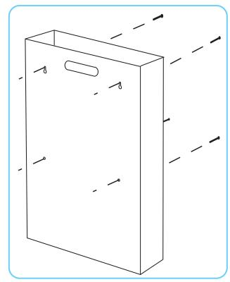
Wall Mount: Securely mount unit to a wall via keyholes and screw holes in back with screws approved and supplied by building maintenance. All four mounting holes provided must be used.
